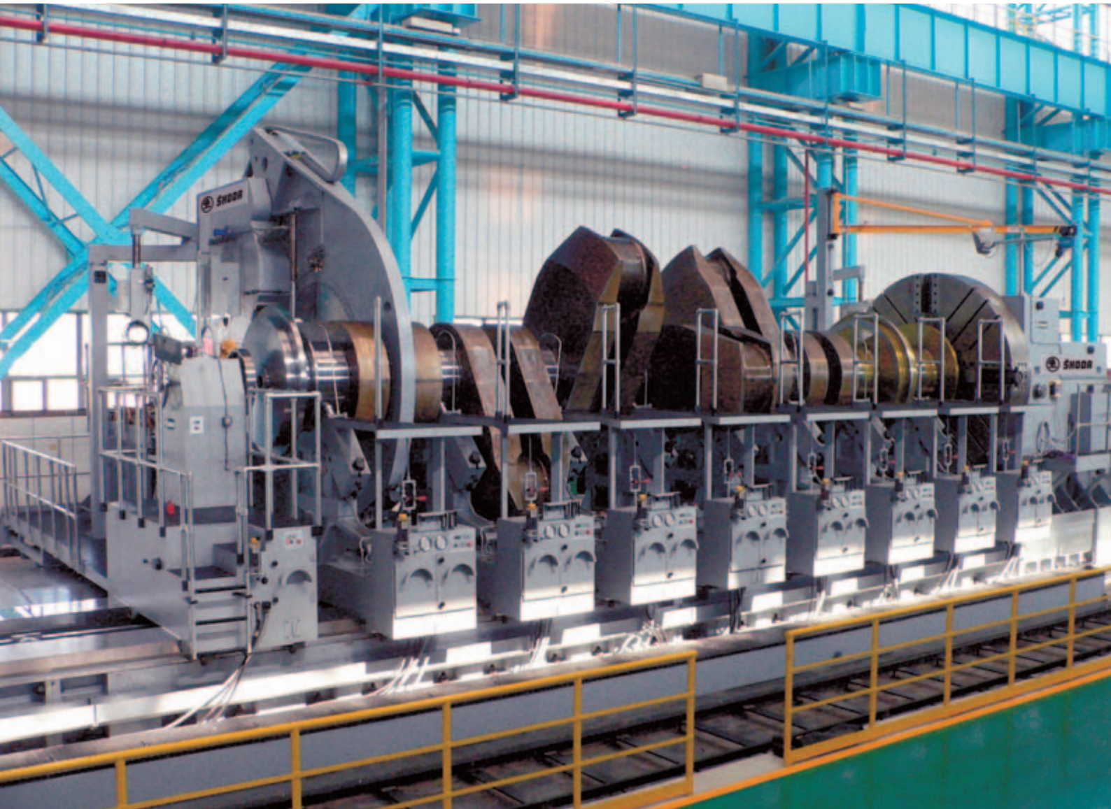
| Special lathe for working crankshafts. Importing country: China. Exporter: ŠKODA MACHINE TOOL, a.s.
